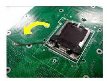
4. Lift the load plate to a fully open position.
